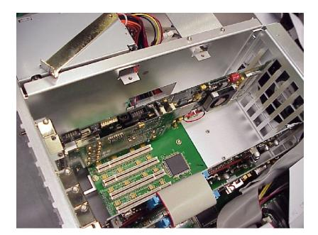
**4.** Press down firmly to engage the module into the connector (see Figure 7).
