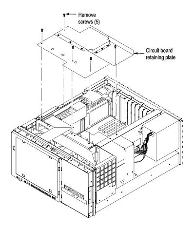
Figure 6: Removing the circuit board retaining plate
