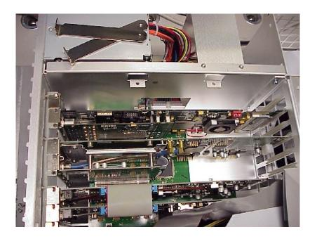
Figure 8: Hardware upgrade module installed in slot 4
