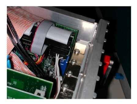
Figure 9: Interface cable connected to controller board
