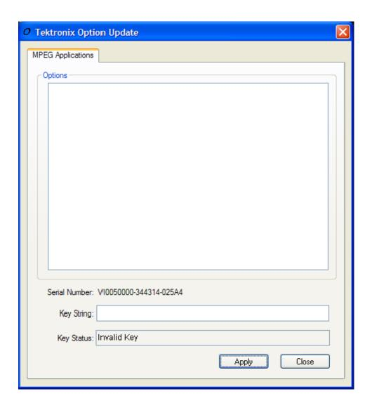
Figure 3: Tektronix Option Update Wizard - Initial view
